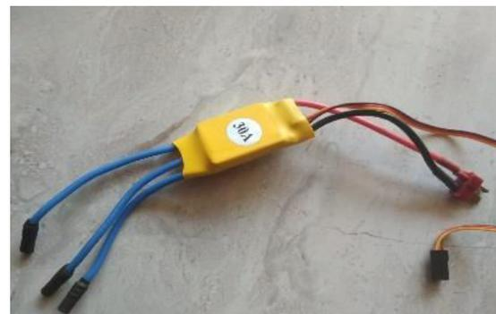
**FIG: ESC (Electronic Speed Controller)**
